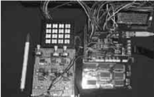
Figure 2: Devised urodynamic study system
